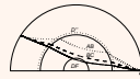
Figure 2 : Ray paths of the three PKP branches in the Earth : PKP(DF) (full line), PKP(BC) (dashed line) and PKP(AB) (dotted line). The event (black star) and the D'' layer at the base of the mantle are also indicated.
